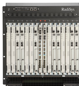
Figure 9. Radisys Promentum® ATCA application-ready platforms for BGF, SBC, and video optimization applications
