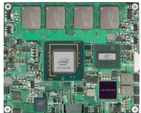
Fig. 4: RadiSys Procelerant Z500 85mm x 70mm board compatible with Type 2 COM Express pinout
